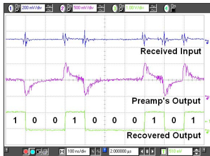
Fig. 6. Measured timing diagram of the AFE at 10-Mb/s.
