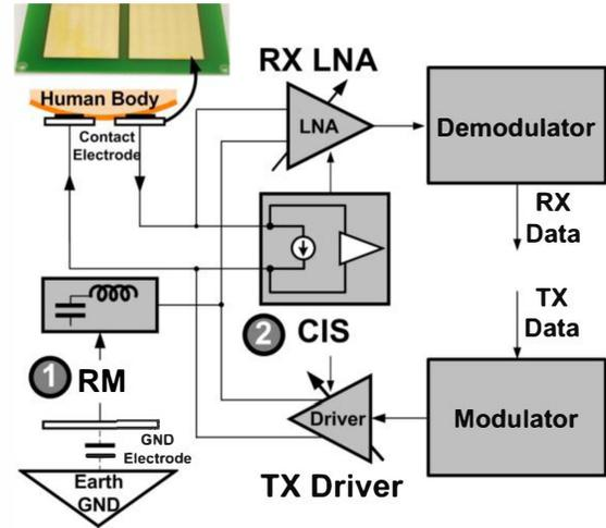
Fig. 9. Energy-efficient transceiver architecture.
