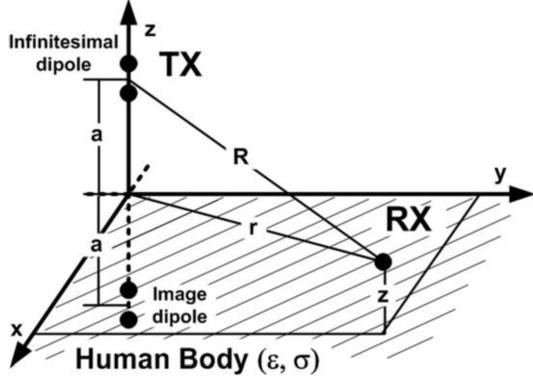
Fig. 1. Electric field from dipole and its geometry on the human body.
