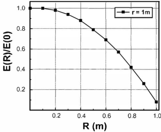
Fig. 7. Effect of the distance between body and contact electrode.
