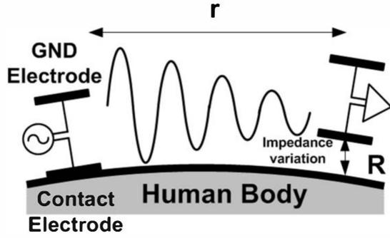
Fig. 6. Surface wave propagation mechanism.
