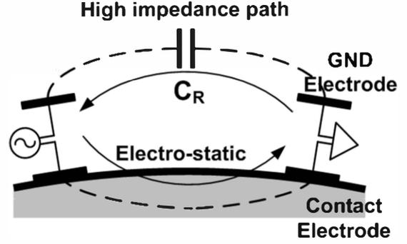
Fig. 4. Quasi-static coupling mechanism.
