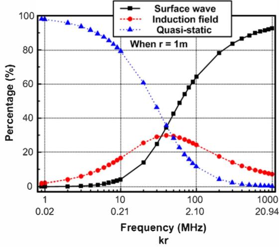
Fig. 3. Contribution ratio of each mechanism in terms of frequency.
