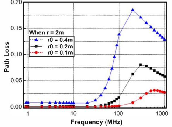
Fig. 2. Frequency response using theoretical analysis.
